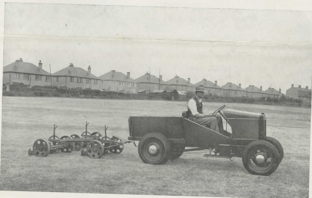
Re-built Triple Mower and Light Tractor at Swansea Corporation Playing Fields
